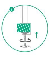
Tighten the bracket clamp from beneath by turning the adjuster clockwise and make sure it's tight. Slide the base cover on and clip into place.
