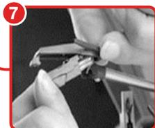
7 Carefully slide the cartridge into the cartridge holder.
