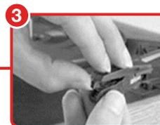
3 Separate the cartridge holder from the cartridge by loosening the locker.
