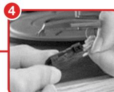
4 Gently pull the audio-lines from the cartridge, pull from the terminal connector and not the wire itself.
