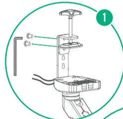
1 Loosen the two screws that connect the two parts of the clamp.
