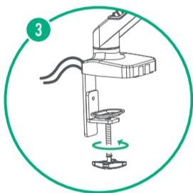
Tighten the securing bracket by turning the adjuster clockwise and make sure it's tight. If your desk is too thick, adjust the clamp down a notch and re-tighten.
