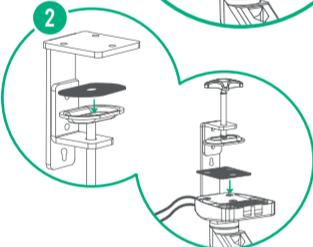
Adhere the bracket cover and the bracket clamp cover to the support block of the bracket clamp.
