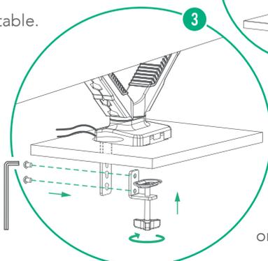
3 Install the lower part of the clamp with the two screws. Tighten the clamp until it is securely fastened to the desk.
