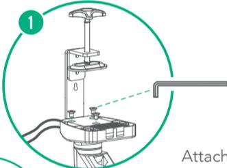
Attach the bracket clamp to the base with the 3 cap screws. Use the 4mm hex key to tighten.
