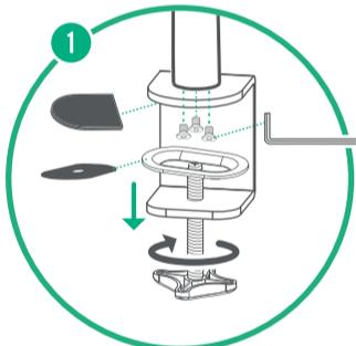
Adhere the bracket clamp cover to the bracket clamp and attach the clamp to the base with the cap screw. Use the 4mm hex key to tighten.
