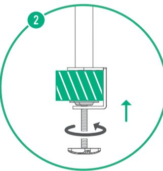
Tighten the bracket clamp from beneath by turning the adjuster clockwise and make sure it's tight. Slide the base cover on and clip into place.
