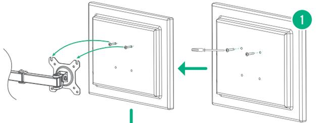
2 Install the lower two screws. Now you can fasten the upper two screws all the way.
