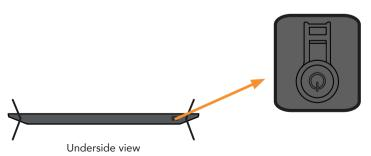
When the TV is on, press and hold button for 1.5 seconds to put TV on standby.
