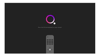
During the first time setup process, when the screen shown above appears, point the remote control towards the IR sensor of the TV and press the **SCROLL WHEEL/OK** button to pair the remote.
